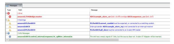
31. To fix this error, change the sequencer\_ser base address to 200. Click on the base value of 0x000 0000 and change the value to 0x0000 0200. The error will go away.
