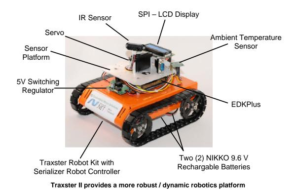
The LCD display provides an on board indicator of the robots current activities. When the robot stops for an obstacle, a temperature reading is made and the result is displayed on the display.
